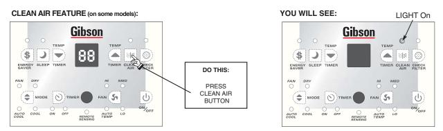
Note: When this feature is "ON", the electronic air purifier is energized to remove pollen and impurities from the air. To cancel this feature, press the Clean Air button (the LIGHT will turn off).
